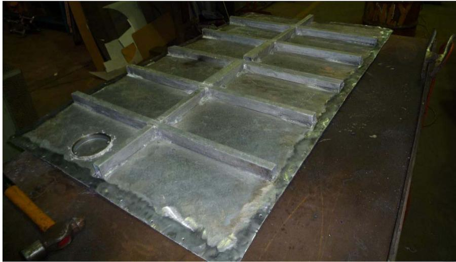
**Step 8** – Remove the fuel sender and drain the tank through the sender hole, using a siphone or fuel pump.
