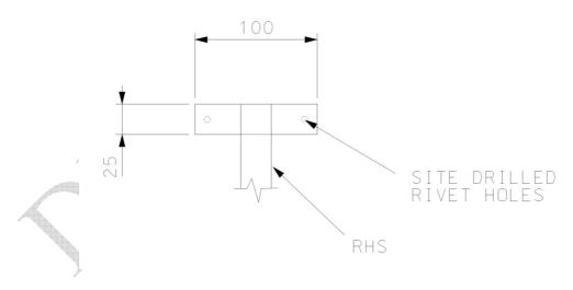
**Step 17** – Cut enough 100mm lengths of RHS to fit under each end of the transverse members
