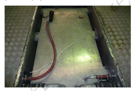
**Step 9** – Remove the fuel lines or loosen them, as they might only come off as the tank is removed.
