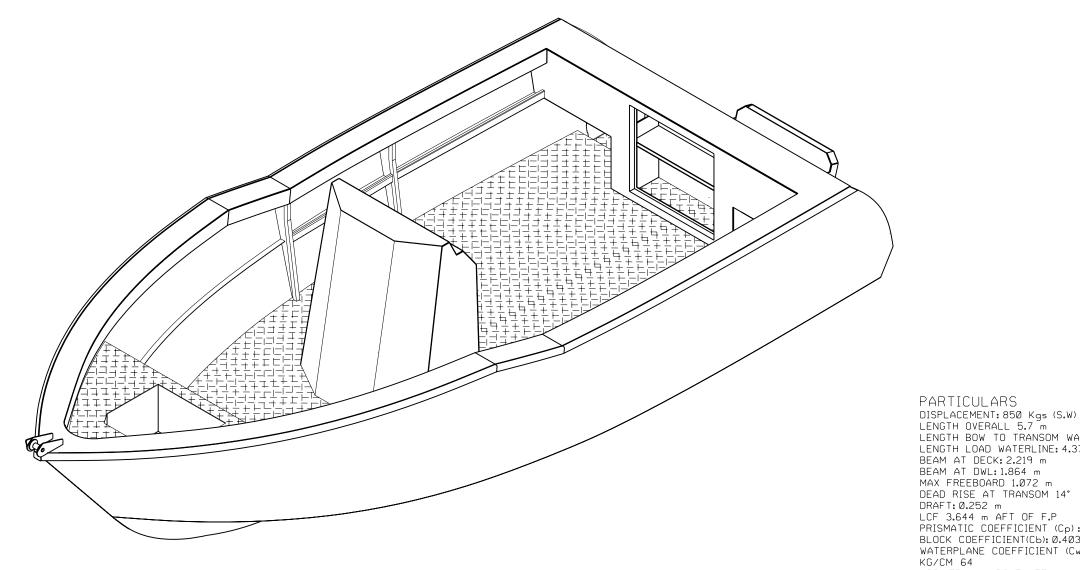
BEAM AT DWL: 1.864 m MAX FREEBOARD 1.072 m DEAD RISE AT TRANSOM 14° DRAFT: 0.252 m LCF 3.644 m AFT OF F.P PRISMATIC COEFFICIENT (Cp): 0.704 BLOCK COEFFICIENT(Cb): 0.403 WATERPLANE COEFFICIENT (Cw): 0.763 KG/CM 64 KG/CM 64
